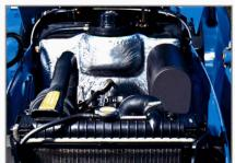
**Large fuel tank** 6.6 gal. capacity provides long operation time
